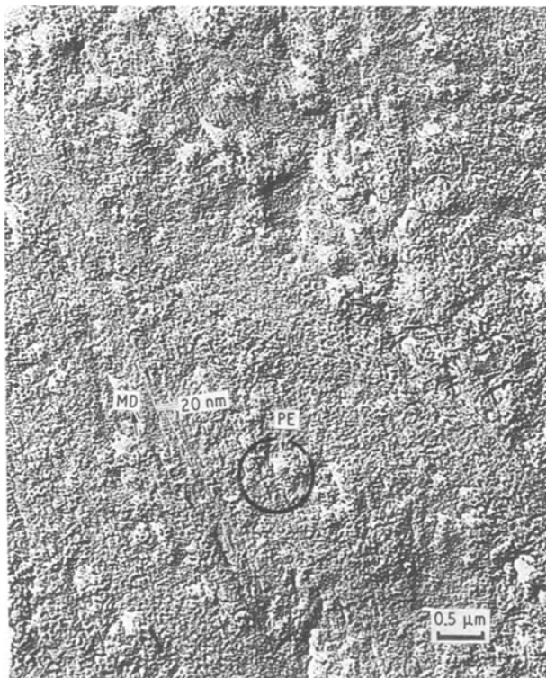
Figure 8 Fracture surface morphology of the XZ plane of the rolltruded copolymer A for T_p = 150^\circ\text{C} , DR = 3.3.
